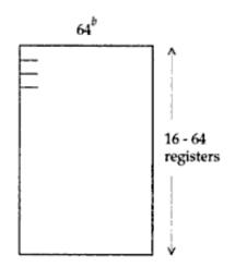
Figure 7.3 Typical vector register sizes.
