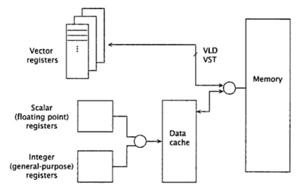
Figure 7.2 The primary storage facilities in a vector processor. Vector LD/ST usually bypasses the data cache.
