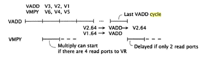
**Figure 7.6** For logically independent vector instructions, the number of access paths to the vector register set and vector units may limit performance. If there are four read ports, the VMPY can start on the second cycle. Otherwise, with two ports, the VMPY must wait until the VADD completes use of the read ports.
