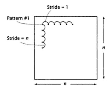
Figure 7.1 For an array in memory, different accessing patterns use different strides in accessing memory.
