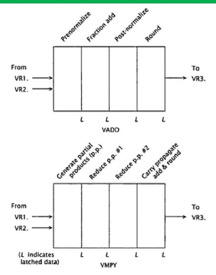
Figure 7.5 Two vector arithmetic units, each partitioned into four pipeline stages. Results are latched at each latch point (*L*).
