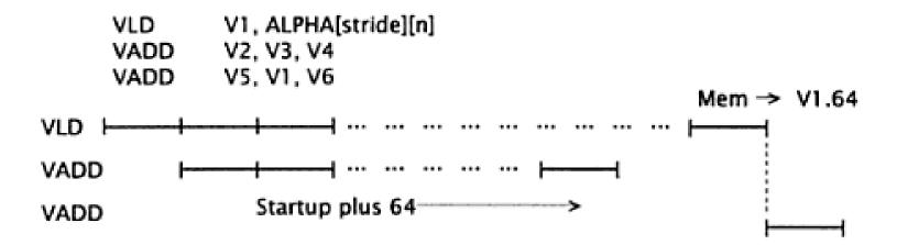
Figure 7.7 While independent VLD and VADD may proceed concurrently (with sufficient VR ports), operations that use the results of VLD do not begin until the VLD is fully complete.
