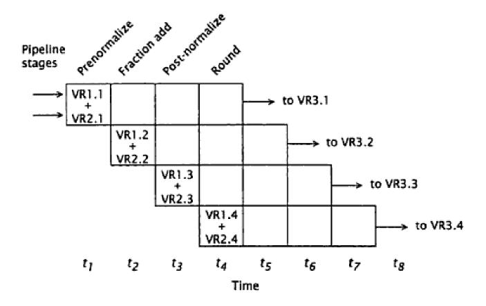
Figure 7.4 Approximate timing for a sample 4-stage functional pipeline.
